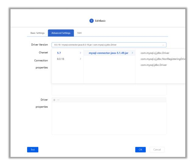
After switching to the custom driver package, click "Test" again to ensure the data source connection is normal. Successful test means the driver package has been successfully changed, click OK, return to the main window, and it can be used normally. The method to add other database drivers is the same as above.
