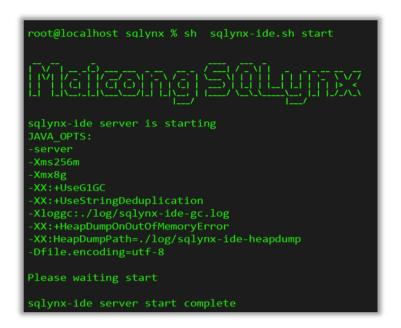
6. After starting, you can access the SQLynx web page by using a browser to navigate to http://<server IP address>:18888. The default port is 18888, and it supports customization.
